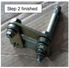
3) Install the shifter shaft ASSY finished above to transmission. (See Figure 74)
