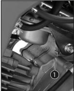
Choke 1 is fitted on the left side of the carburetor.
