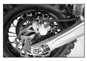
• Manually press the brake caliper toward the brake disc to push back the brake pistons. Ensure that brake fluid does not flow out of the brake fluid reservoir, if necessary extract excess.
