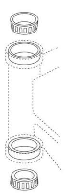
Remove the lower triple clamp. (1.56)
