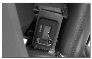
Service hour counter 1 is fitted in front of the handlebar.
