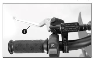
The Handbrake lever (rear) 1 is located to the left of the handlebar.
