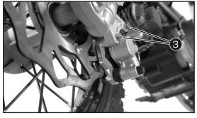
• Position the brake caliper, put the screws 3 in place and tighten.
