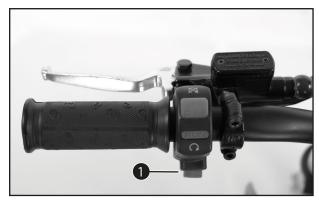
Electric starter button 1 is fitted on the right side of the handlebar.
