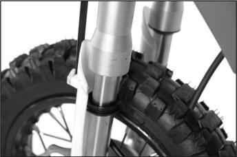
The dust-protection bellows 1 are to remove dust and coarse dirt particles from the fork tube. However, after some time, dirt may also get in behind the dust-protection bellows. If this dirt is not removed, the oil sealing rings located behind it may start to leak.
