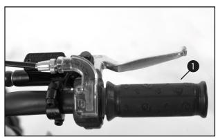
The throttle grip 1 is fitted on the right side of the handlebar.
