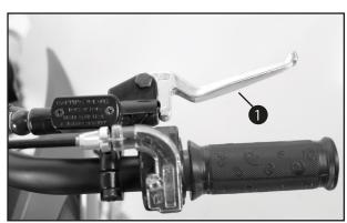
Handbrake lever (front) 1 is located on the right handlebar. The front brake is operated by the handbrake handle.
