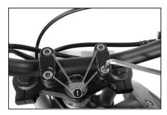
For this purpose, remove screws 1 of the handlebar clamps. Mount handlebar and handlebar clamps, and tighten screws 1 to 29 Nm. The gap between the handlebar support and handlebar clamps should be the same size in the front and in the rear.
