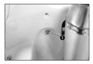
• Remove the screw 1 bellow the seat
