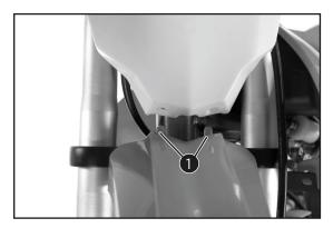
• Position the fender with drill holes 1 in the holding lugs on the start number plate.
