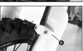
• Position the brake line and clamp. Mount and tighten screws 7.
