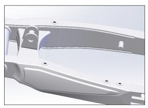
Check the swingarm for damage, cracking, and deformation.
