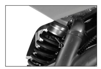
The spring preload can be changed by turning the adjusting ring 1. For this purpose, you should dismount the shock absorber and clean it thoroughly.
