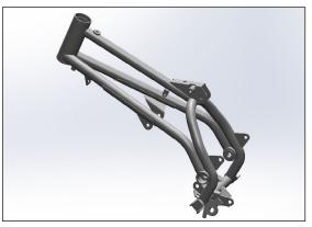
• Check the frame for cracks and deformation.
