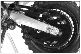
• Check the chain sliding guard for wear.
