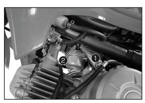
• Screw in the idle adjusting screw 2 until it stops and then to the prescribed basic setting.
