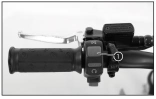
Kill switch 1 is fitted on the left side of the handlebar.
