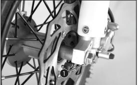
Check the wheel bearing for damage and wear.
